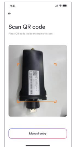
3. Scan WiFi stick QR code or manually enter the serial number and the registration code
