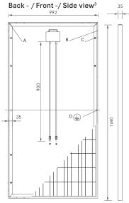
A: 4 x drainage 10\*10 mm B: 8 x ventilation aperture 3\*7 mm
