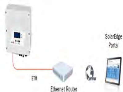
Figure 6: Single device Ethernet connection
