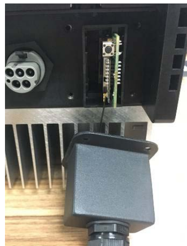
Fig. Insert the GPRS card
