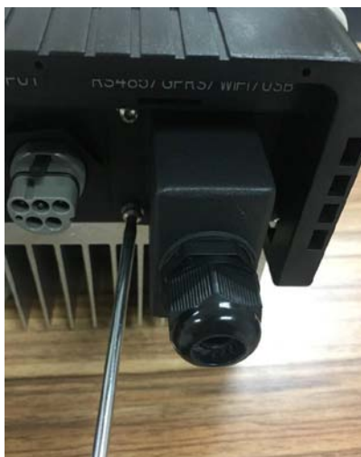
Fig. Dismantle the communication box
