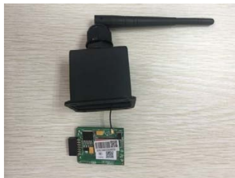
Fig. Connect the GPRS antenna
