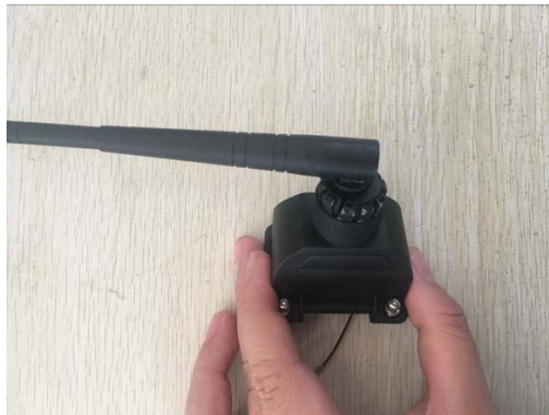
Fig. Insert the GPRS antenna
