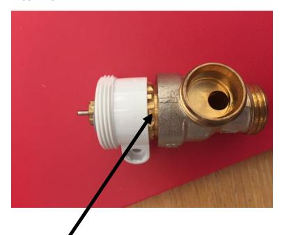
MIND the GAP (when fitting the Adaptor clip ..spread the clip further open & locate hard against the body see below.
