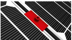
Alternatively: Use two XS middle clamps between two modules. Insert the MK2 nut into the mounting rail and turn clockwise by 90 °. Place clamps on the module frames and fix them.
