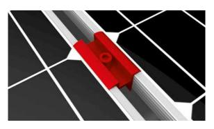
Use two universal module middle clamp OneMid between two modules. Klick the Stance in the notches. Place clamps on the module frames and fix them. Make sure that the terminals are always mounted centrally on the rail (MultiRail 10 and 25!).
